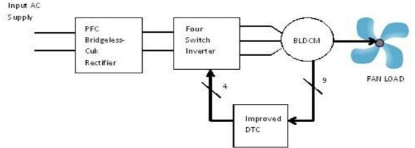
Fig. 1 Block diagram of the proposed system.
