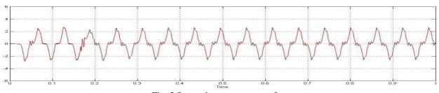
Fig. 5 Stator phase current waveform.
