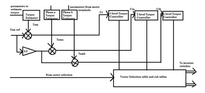
Fig. 2 Block diagram of the improved DTC
