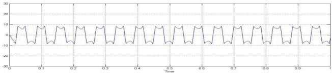
Fig. 6 Back EMF waveform.
